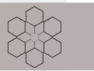
The frame is designed to securely hold 6 TIPA products, each weighing 1.7 kg. It features a central nylon bush, which helps to reduce friction and wear at the joint. The solar products are fastened to the frame using stainless steel fasteners, ensuring stability and resistance to corrosion.
